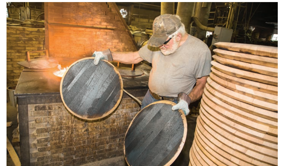
Charring the barrel affects the tannins in the oak, which provide hints of vanilla, butter, and spice to the bourbon, while the charred interior gives it an amber hue.
