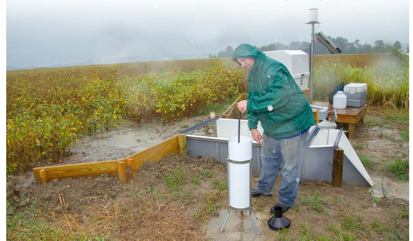
Mark Akland measuring runoff during a rain event.
