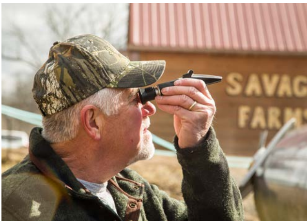
Using a refractometer, Keith Moore checks the sugar content of the maple sap in his holding tank at his Savage Farms in Lawrence County.
