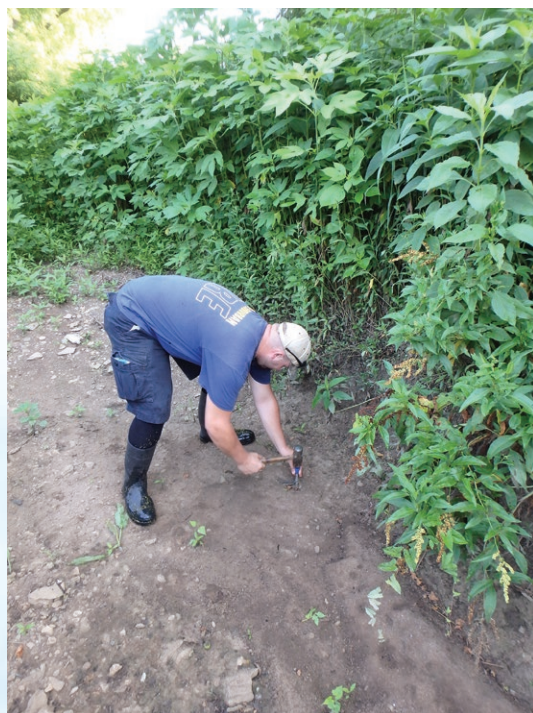
Chris Sass measures erosion by planting pins along the banks of Cane Run Creek in northern Fayette County.
